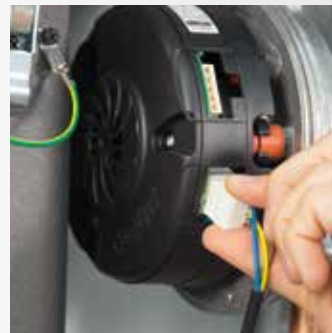
Removal of the fan harness
